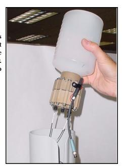
Figure 5-36. Installing the EGC in the Holder
