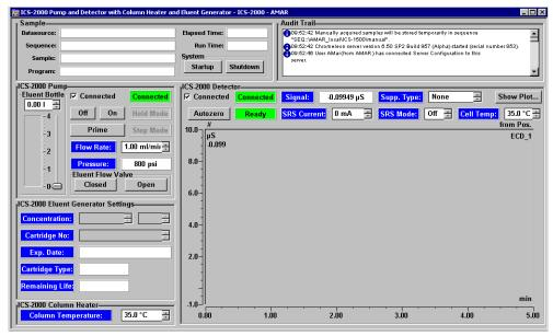
Figure 2-12. ICS-2000 System Control Panel (Traditional)
