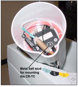
Figure B-28. Cartridge Holder (tilted to view the bottom)
