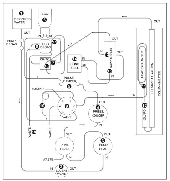
Figure 5-7. ICS-2000 Flow Schematic
