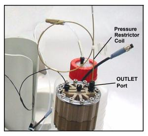
Figure B-38. EGC Outlet Connection for Conditioning the EGC
