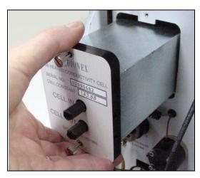
Figure 5-16. Removing the Cell Assembly
