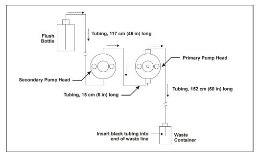
Figure B-69. Piston Seal Wash Flow Schematic
