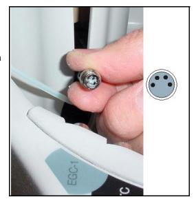
Figure 5-37. Connecting the EGC Cable
