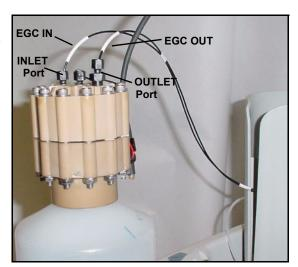
Figure 5-38. EGC Inlet and Outlet Connections
