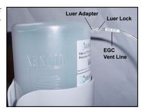
Figure B-42. Installing the EGC Vent Line
