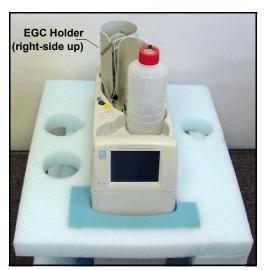
Figure B-2. ICS-2000 After Installing Eluent Bottle and EGC Holders
