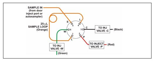
Figure 3-12. Injection Valve Connections
