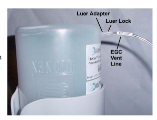
Figure 5-29. EGC Vent Line and Luer Fitting
