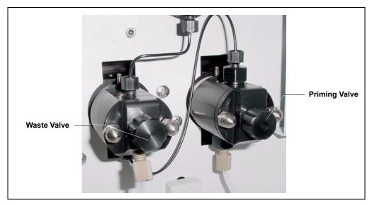
Figure 5-13. Waste and Priming Valves
