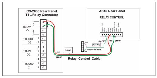
Figure B-65. Example AS40 Autosampler Connection
