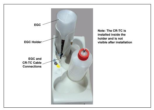
Figure B-26. ICS-2000 with an EGC Installed (Top View)
