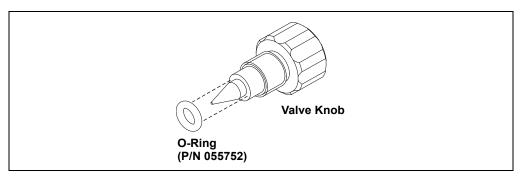
Figure 5-14. Waste Valve or Priming Valve O-Ring Replacement
