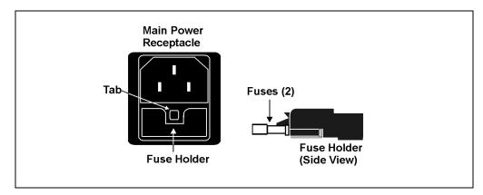
Figure 5-28. Main Power Fuse Holder
