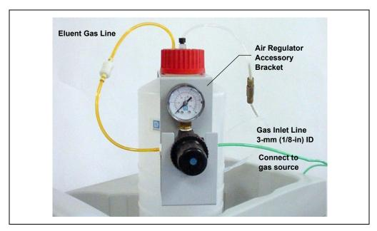
Figure B-67. ICS-2000 Pressurized Eluent Reservoir Connections (Optional)
