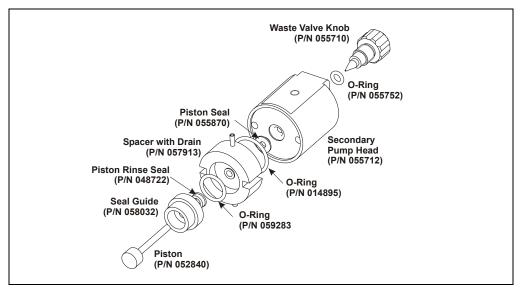
Figure 5-12. Secondary Pump Head
