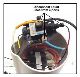
Figure 5-40. Disconnecting CR-TC Liquid Lines
