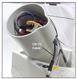
Figure B-32. Installing the CR-TC
