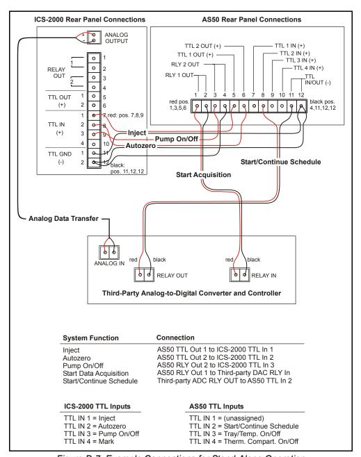
Figure D-7. Example Connections for Stand-Alone Operation
