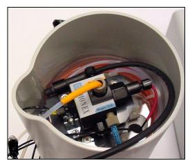
Figure 5-41. CR-TC Installed in Holder
