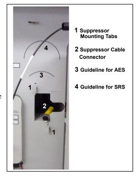
Figure B-19. Suppressor Mounting Tabs and Guidelines
