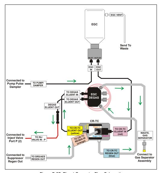
Figure B-27. Eluent Generator Flow Schematic
