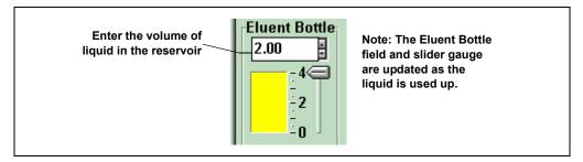
Figure 3-8. Chromeleon Control Panel: Setting the Eluent Level
