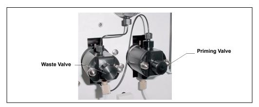
Figure 4-2. Waste and Priming Valves
