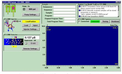
Figure 2-13. ICS-2000 System Control Panel (Graphical)
