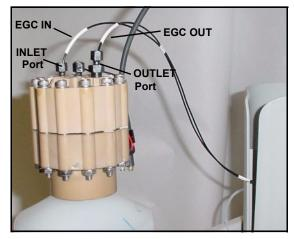
Figure 5-49. EGC Inlet and Outlet Connections
