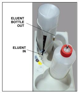
Figure 3-10. Reservoir Connections
