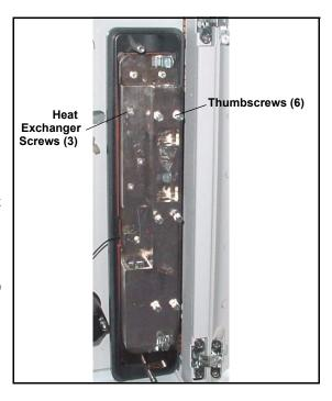
Figure 5-22. ICS-2000 Column Heater Cover Removed
