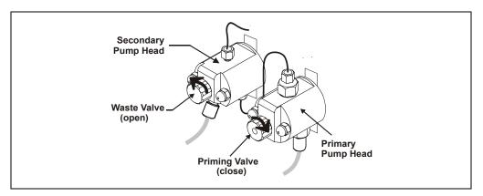
Figure 3-11. Priming the Pump
