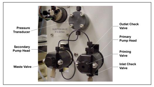
Figure 2-16. ICS-2000 Pump Components
