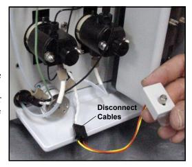
Figure 5-27. Leak Sensor Cable
