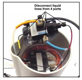
Figure 5-45. Disconnecting CR-TC Liquid Lines
