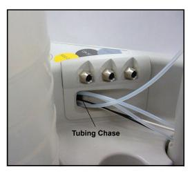
Figure 5-44. Top Cover Tubing Chase
