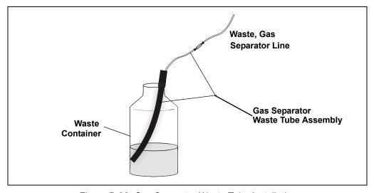
Figure B-22. Gas Separator Waste Tube Installation
