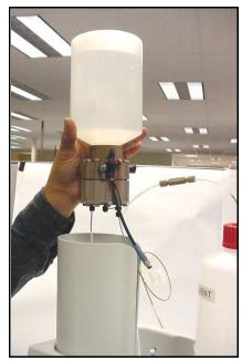
Figure B-39. Installing the EGC in the Holder
