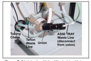
Figure B-61. Injection Valve Waste Line Union
