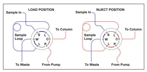
Figure 2-17. Injection Valve Flow Schematics
