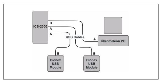
Figure B-8. Example Connections: Two Dionex USB Modules Connected to the ICS-2000
