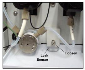
Figure 5-26. Leak Sensor
