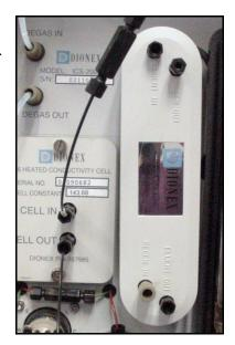
Figure B-20. Suppressor Installed (SRS Shown)
