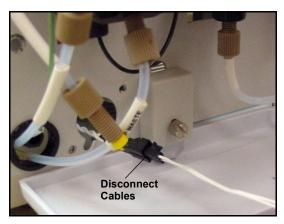
Figure 5-24. Eluent Valve Cable
