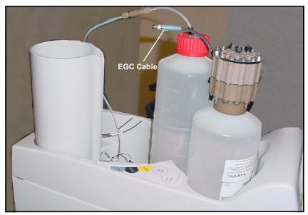
Figure B-36. EGC Cable Orientation
