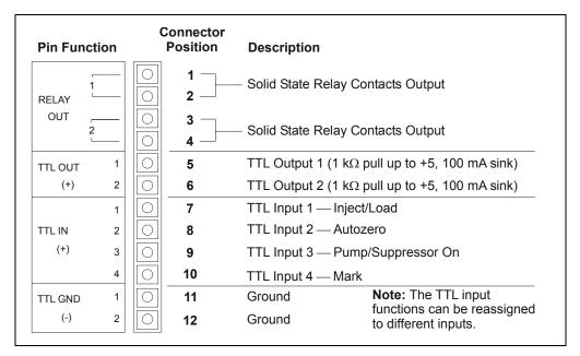
Figure D-1. TTL and Relay Connector on Rear Panel
