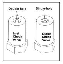
7. Install the inlet check valve assembly (P/N 045722) on the bottom of the primary pump head. Install the outlet check valve assembly (P/N 045721) on the top of the head. Tighten the check valves fingertight, and then use a wrench to tighten an additional one-quarter to one-half turn.
