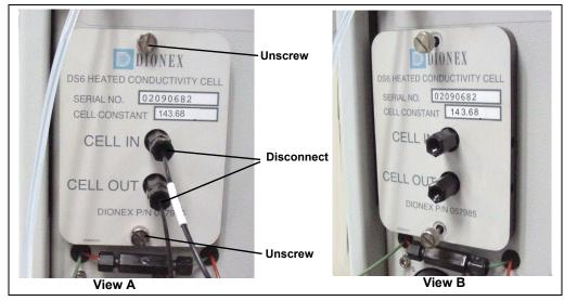
Figure 5-15. Removing the Cell Front Cover
