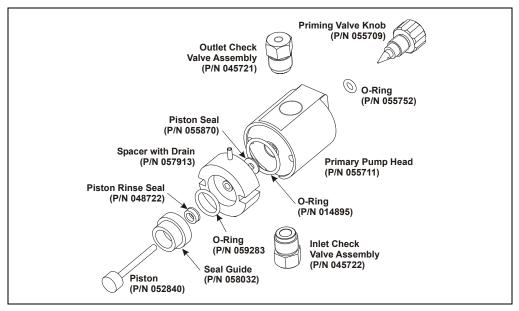
Figure 5-11. Primary Pump Head
