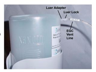
Figure 5-43. EGC Vent Line and Luer Fitting
