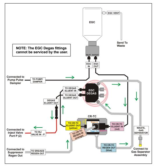
Figure 5-8. Eluent Generator Flow Schematic
