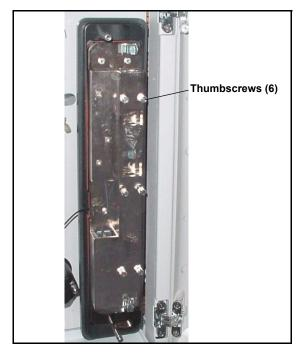
Figure 5-20. ICS-2000 Column Heater Cover Removed
