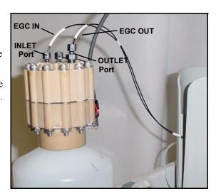
Figure 5-32. Disconnect the Inlet and Outlet Port Lines
