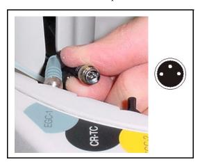
Figure B-44. Connecting the CR-TC Cable
