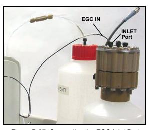
Figure B-37. Connecting the EGC Inlet Port
