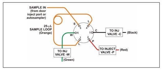
Figure 2-18. Injection Valve Plumbing
