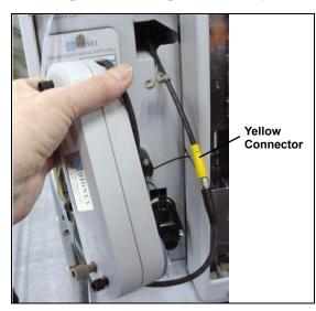
Figure 5-18. Removing the Suppressor
