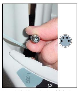
Figure B-40. Connecting the EGC Cable
